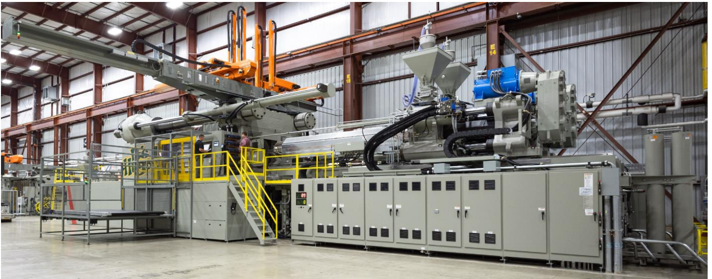
The C8000 spans 94-feet in length, weighs 1.8 million pounds, and contains nearly 38 miles of wire.
